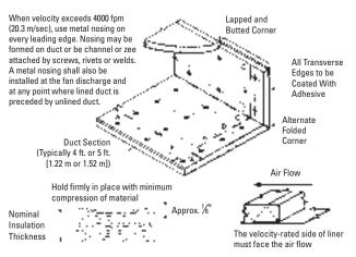
Liner adhered to the duct with 90% min, area coverage of adhesive. Adhesive shall conform to
